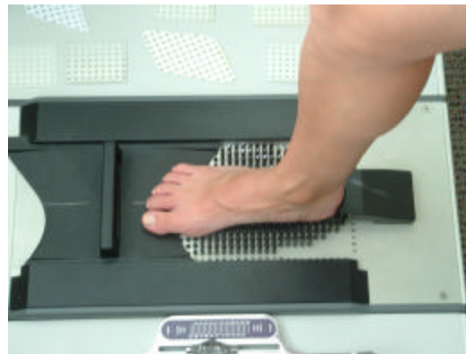
Digital mapping of biomechanical corrections to your foot and ankle in order to produce your custom orthotic.
